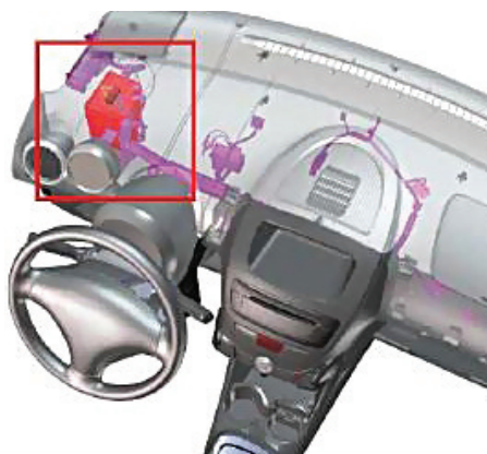
The EPS can be accessed by removing the top of the dash
