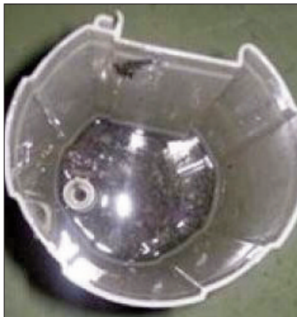
Paint sludge inside the fuel pump assembly
