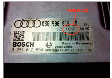
The ECU type can be read of the label
