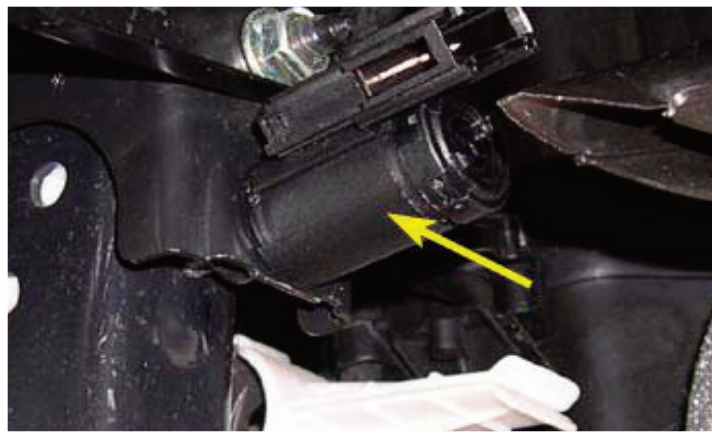
Fig. 2 The brake pedal switch installed on the pedal assembly
