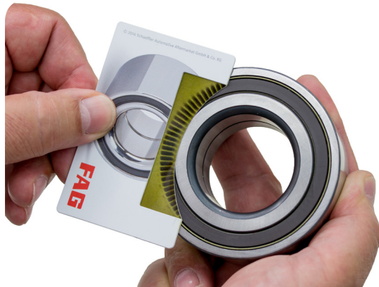
Fig. 1: The encoder card can be used to determine the installation side of a multipole encoder. With passive encoders, this does not work.
