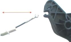
The end fitting housing must be perfectly clean before fitting the cable to the pedal
