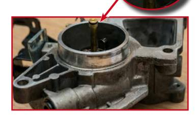
Please check the rubber seal on your brake vacuum pump (see photo) which creates a seal within the camshaft oil feed journal.
