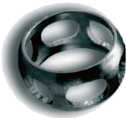
Deformation of the surfaces on this bearing cage would require the CV to be replaced
