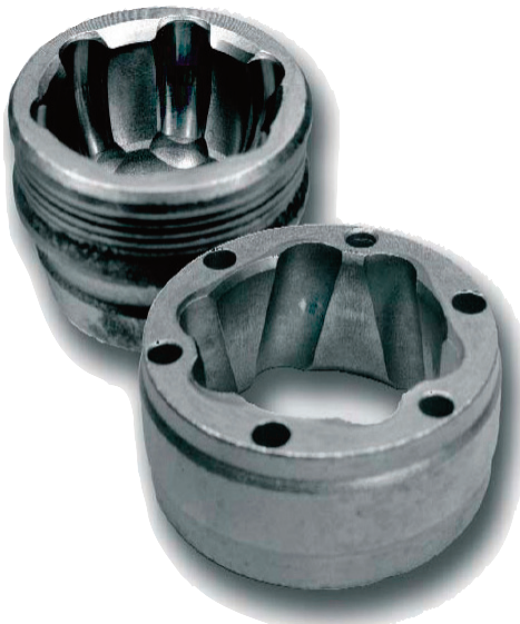
Examine the interior of the CV joint for any wear, beyond polishing
