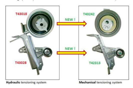
This new idler bracket T42313 is of almost exactly the same design as the previous vibration damper T43028, but <u>without</u> the hydraulic element - it's only a metal bracket with a small touch idler.
