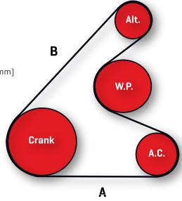
**Break-in Procedure:** Recommended drive cycle is no less than 20 minutes before checking and setting final drive tension.
