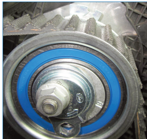
Figure 2 - The OE T43219 tensioner supplied by Gates for the same engines as Figure 1
