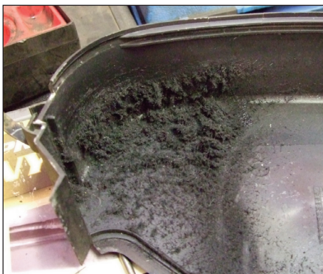
Debris from the worn belt was abundant inside the drive system cover
