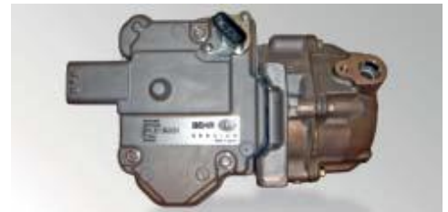
The high-voltage compressor
