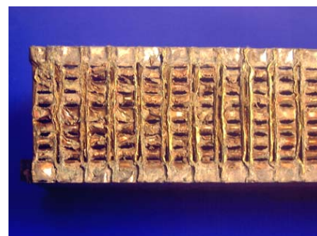
Poor performance caused by deposits
