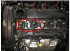
If the water rises up to the spark-plug connectors, arcing and, therefore, misfires occur. In this case, the spark-plug connectors and ignition coils must be removed and the shafts purged using compressed air.
