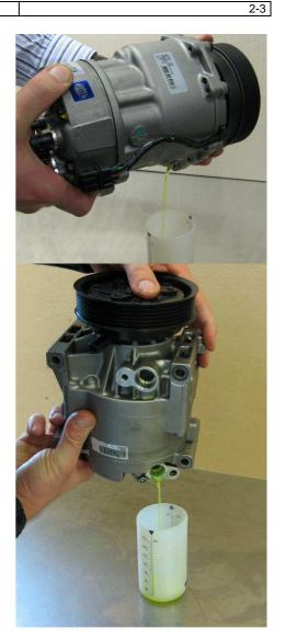
e.g. without filling bore hole through the high-pressure connection
