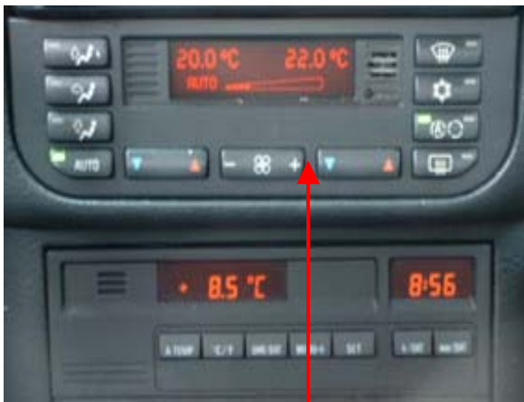
Climate control panel
