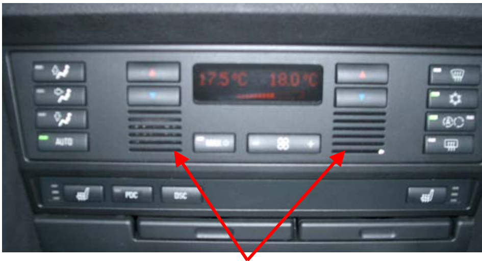
Blower for interior temperature sensor
