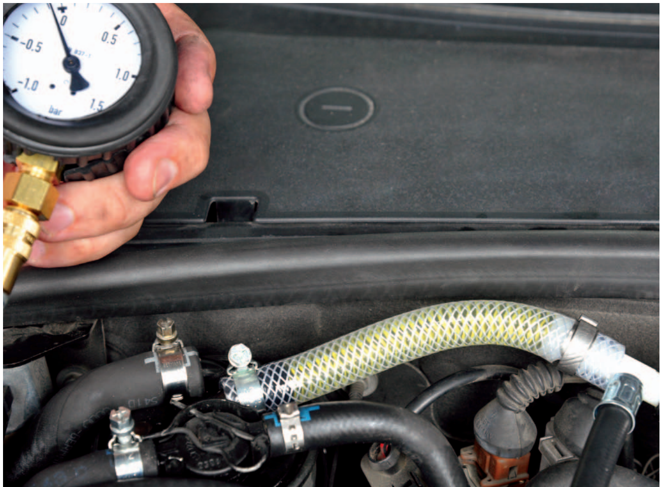
Bubbles or foaming may not be detected in the distributor-type injection pumps controlled by solenoid valves in the fuel system. A transparent hose is looped into the fuel supply for the test.
