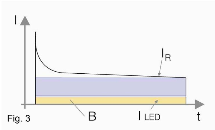
In this case, only a flasher unit according to principle c would work. If the resistance is chosen somewhat higher, principle d could also possibly work. If the light then fails due to mechanical damage, the flasher unit could detect the inserted resistor as a functional bulb. In this case, a light working perfectly would be indicated although this is not the case! This means: In this case the vehicle would lose its approval for use on public roads.
