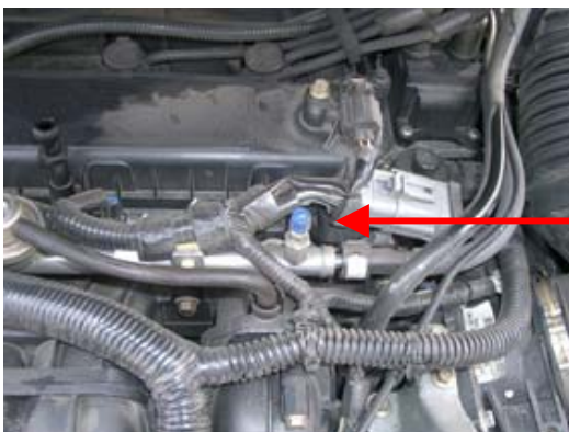
Connection for testing fuel pressure
