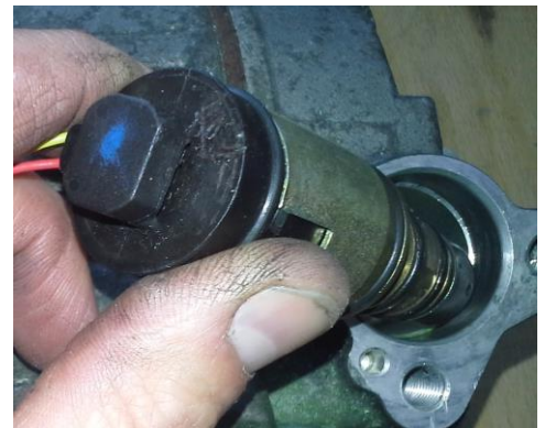
The figure shows an example of an electronically actuated pressure control valve
