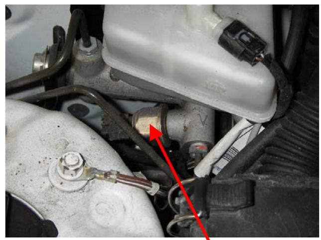
Fig. 4 Brake pressure sensor
