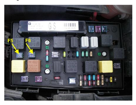
F5 fuse for radiator fan motor 1 F6 fuse for radiator fan motor 2
