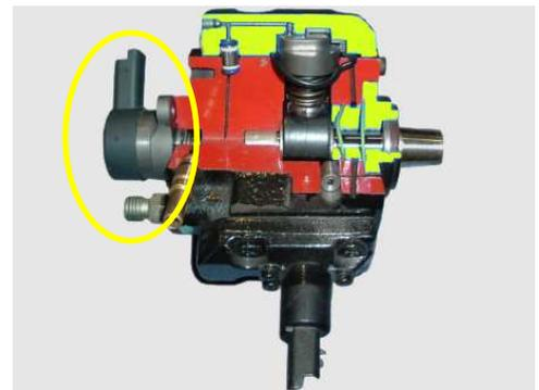
The dosing unit is available as a replacement part, so you do not need to replace the entire high-pressure pump. The unit is extremely susceptible to dirt, so you should take care to avoid any contamination while performing the repair.
