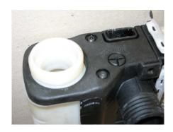
Since the expansion tank is installed in the radiator as a separate component, there is a recess behind it where part of the liquid can collect. This can drain off through an opening on the base of the tank.
