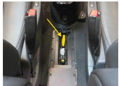
Note: The emergency release/the control element of the electric parking brake will automatically reset to its working position the next time the EPB switch is pressed.
