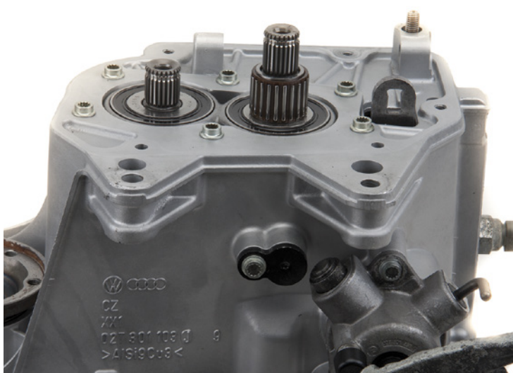
Twin-bearing mounting plate assembly and needle bearings of a 02T transmission
