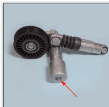
Bolt broken due to excessive side load.
