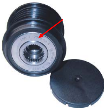
Excessive vibration causing housing to break.
