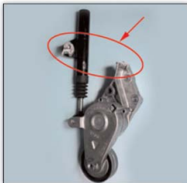
Excessive vibration causing housing to break.
