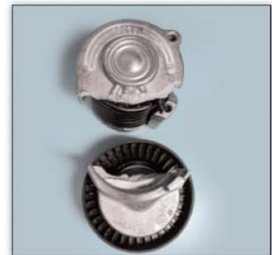
Excessive vibration causing housing to break.
