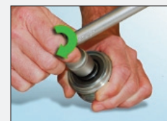
The tool can be continuously turned in a clockwise direction with slight resistance
