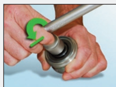
The tool jams immediately and cannot be turned when moved in an anti-clockwise direction.
