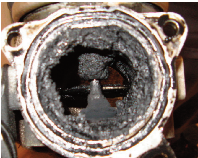
This car was running poorly. The accumulated sludge, varnish and soot obviously would be causing problems.
