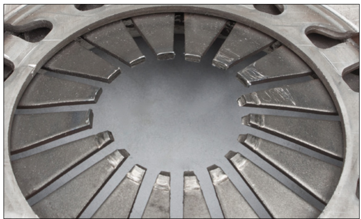
Figure 1: Faulty diaphragm spring caused by lack of preload
