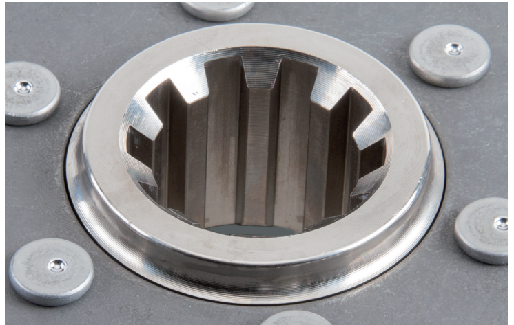
Fig. 1: Nickelled hubs must not be greased
