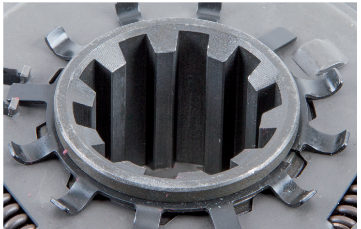
Fig. 2: Phosphated hubs must be greased
