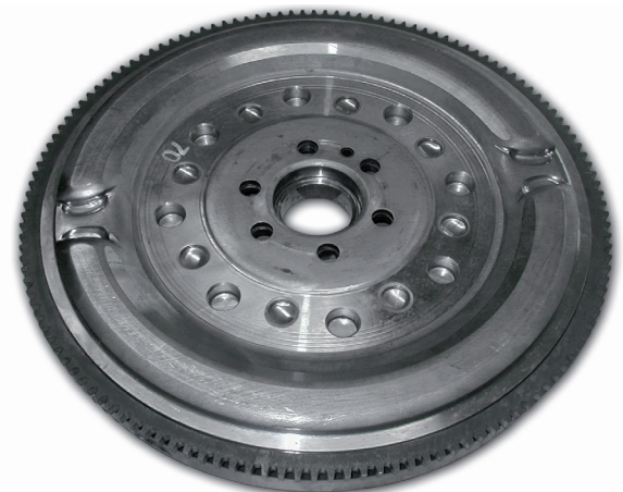
Image 2: SACHS DMF without bead on outer radius
