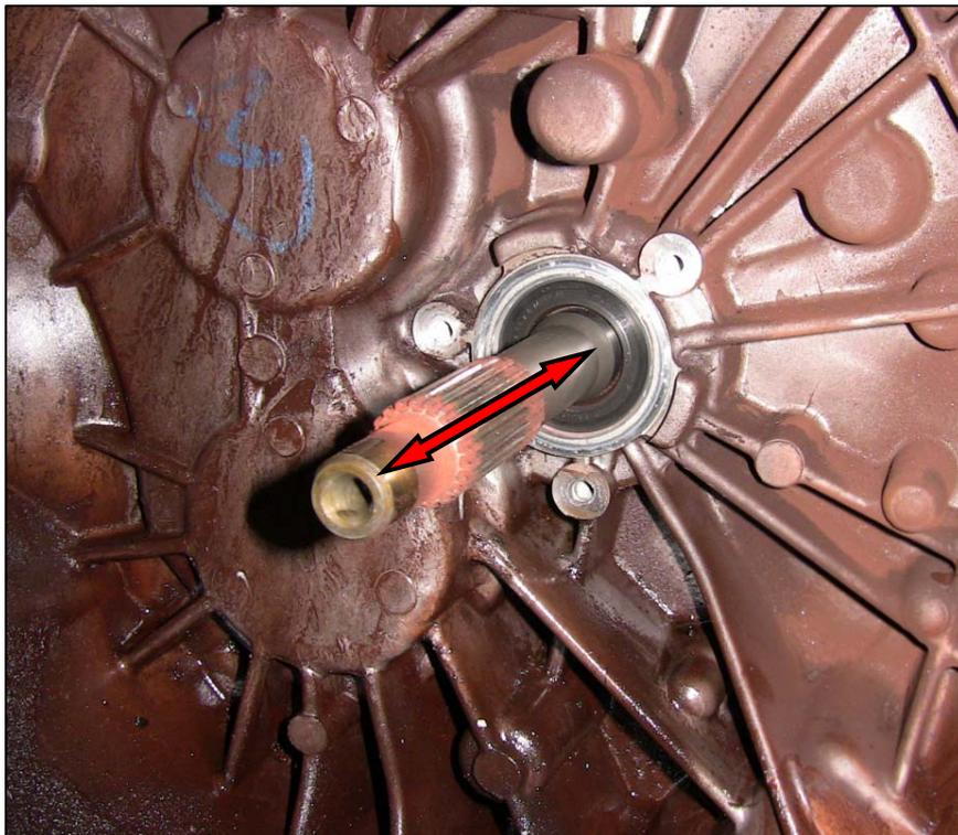
If excessive movement is found then the gearbox must either be overhauled or replaced.
