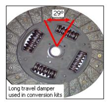
The DMF is designed in such a way as to enable up to 100° of vibration damping as opposed to the 29° from the "Long travel" damper used in the conversion kits.
