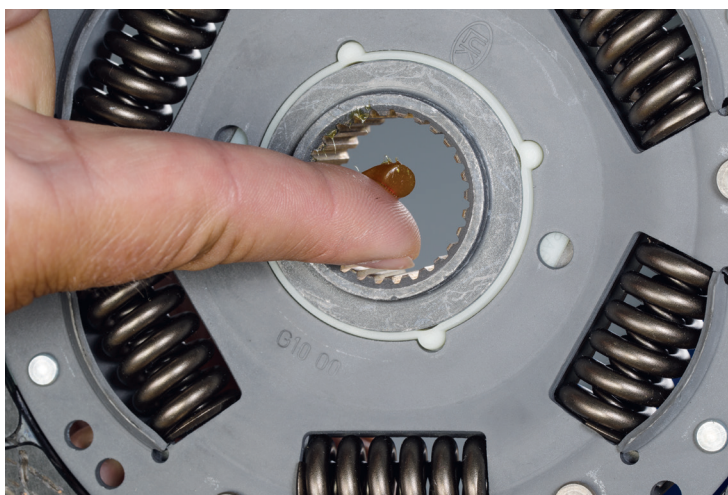
Figure 1: Greasing the hub splines
