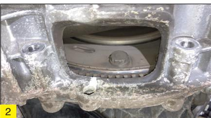
differential by removing the six bolts and remove the centre bearing bracket, which will allow the propshaft to slide away from the differential and hang down.
