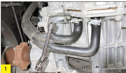
Remove the black plastic blanking cover from the bottom of the bellhousing, this will now give access to the flywheel to drive plate bolts that need to be removed (Fig 2). Remove the three bolts, position a transmission jack under the gearbox to support its weight and remove the gearbox mounting. Disconnect the propshaft from the
