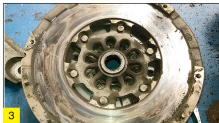
Remove the clutch release arm and bearing assembly to allow the bellhousing area to be cleaned with clutch and brake dust cleaner. Replace the release bearing guide tube supplied in the LuK RepSet clutch kit, mount the new release bearing onto the release arm and refit the release arm.
