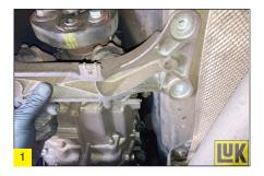
disconnect it from the gearbox flange and position it above. Support the gearbox with a transmission jack, remove the rear gearbox mounting
