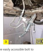
bracket. Leave one easily accessible bolt to secure the gearbox. Ensure the transmission jack is in a central position supporting the gearbox, then remove the final bell housing bolt and ease the gearbox away from the engine. Once clear, lower the gearbox and stow the gearbox safely.
