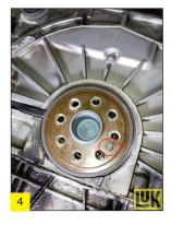
and the release system, so remove the clutch release bearing and release arm, inspect the ball pivot and release bearing guide tube for any wear and replace if required. Clean the bell housing using clutch and brake dust cleaner. Mount the new release bearing and release arm, ensuring the release bearing is positioned correctly, a process that is explained by a nonverbal bulletin that is supplied with the replacement clutch.
