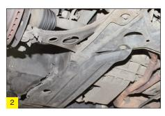
Remove left and right side steering rack to subframe brackets. Remove the steering pump from the subframe by loosening the hexagonal bolt, allowing the pump to slide up from the bracket on the subframe. Undo the wheel arch liner flap on the left hand side, to expose two further bolts and air con pipe bracket to remove. Safely stow the power steering pipes. Detach the steering rack from the subframe, and carefully lower the front of the subframe using 2 axle stands (or rope) as support.
