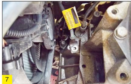
Remove the gear change cables, and stow in the bulk head area. Release and ease the engine wiring loom back from the bell housing area, to gain access to the top bell housing bolts and remove the top bell housing bolts. Raise the ramp and support the gearbox with a transmission jack, before removing the two remaining bell housing nuts and removing the mounting studs using a Torx attachment.
