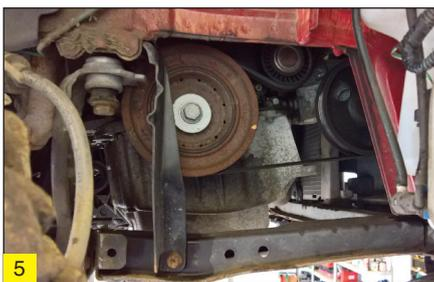
Support the sub-frame, remove the nuts from the additional brackets and the support bolts at the front of the sub-frame. Then lower the front sub-frame and disconnect the lower radiator mountings. Subsequently, the front sub-frame can be removed and stored in a safe location.
