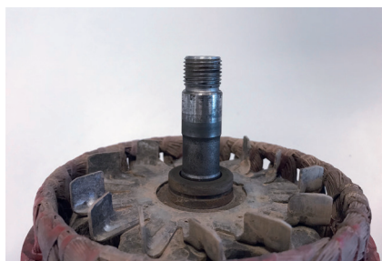
Figure 1: Ground-down shaft in the bearing area
