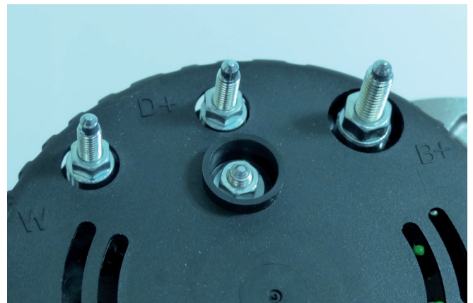
Figure 2: Terminal designation on the alternator: W = speed signal, D+ = battery charge indicator, and B+ = battery plus
