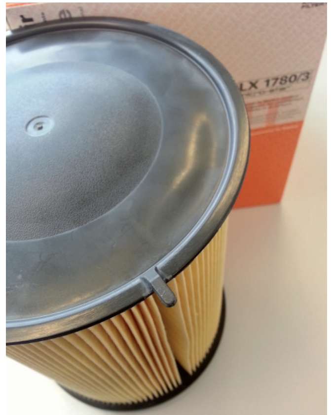
Figure 2: MAHLE LX 1780/3 air filter insert with patented anti-rotation protection
