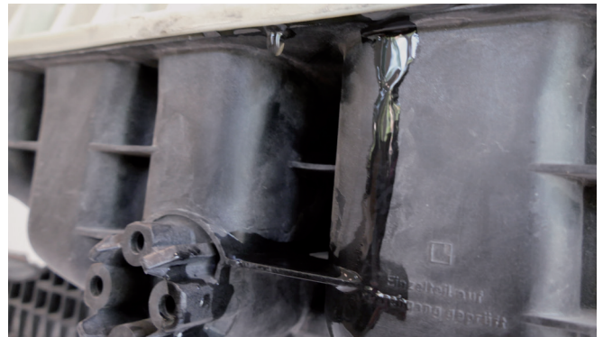
Figure 3: Excess coolant escaping again around the joint face on the expansion tank
