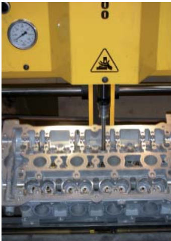
Figure 1: Pressing out of the valve guide
