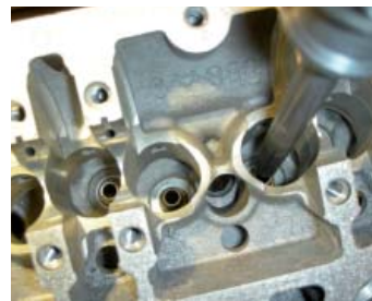
Figure 2: Pressing in of the valve guide
