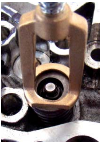
Figure 1: Springing of the valve
