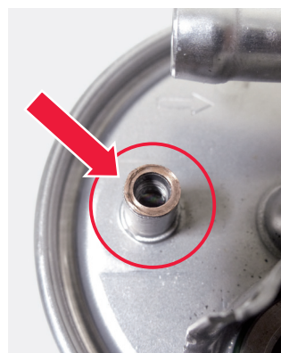
Figure 2: Sealing of the drain screw on the diesel fuel filter KL 154.
