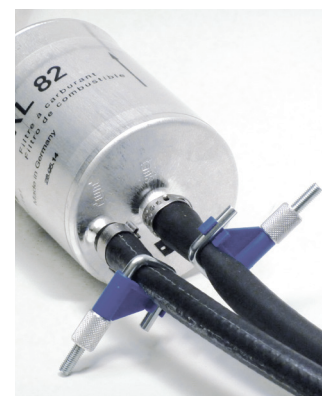
Figure 3: Pinching off the lines prevents air from penetrating into the fuel system.
