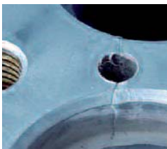
Figure 5: The cracked partition – result of excessive overlap.
