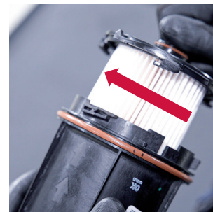
Figure 2: The variant with a brown seal has a bayonet lock
