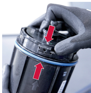
Figure 1: The filter with the blue sealing ring should be aligned and then pressed down until it snaps into place
