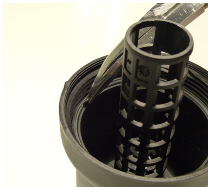
Figure 2: The spring fixing plate can be used to remove the old gasket
